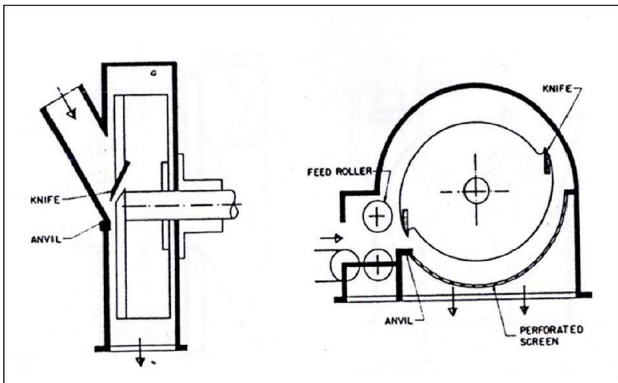
Figure 17. Schematic of the wood-chipper drum
