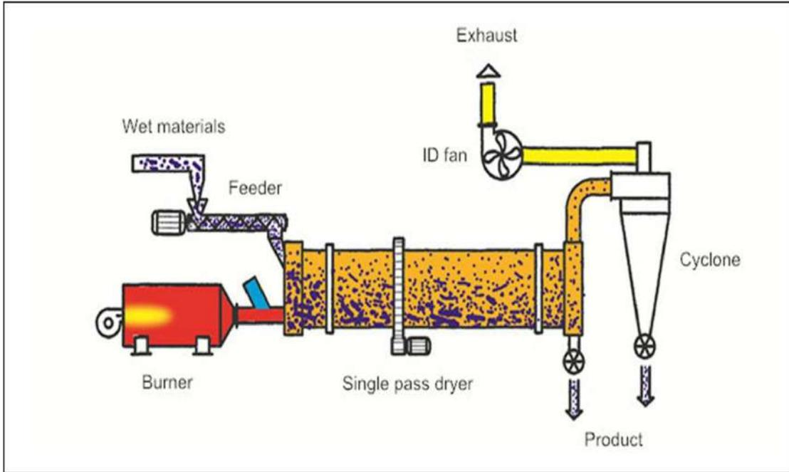
Figure 18. Schematic of the chips drying machine
