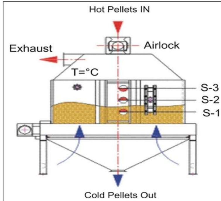
Figure 23. Counter flow cooler
