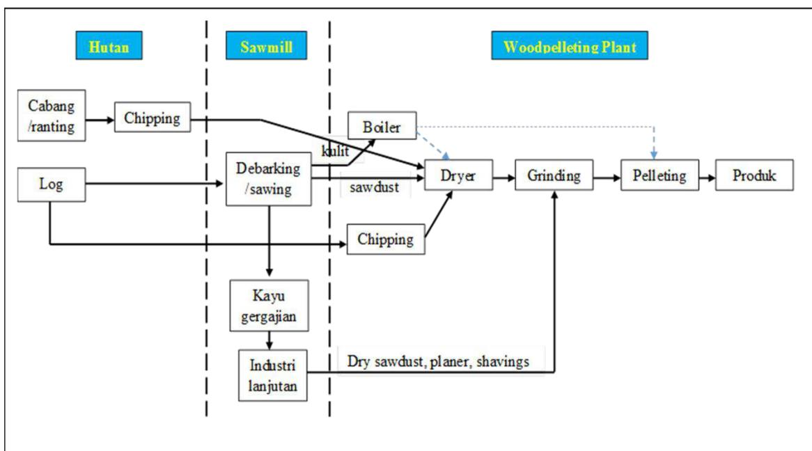
Figure 16. Wood pellet production process
