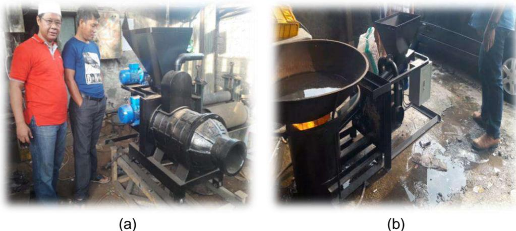
Figure 26. Wood pellet stove, (a) Horizontal, (b) Vertical
