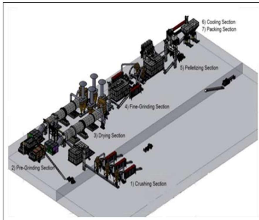
Figure 25. Lay out of Wood Pellet Mill Capacity of 10 Tons/hour (Yulong, 2019)
